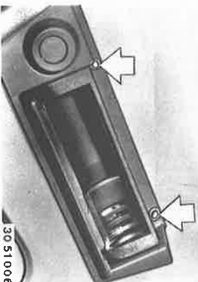
Unscrew bolts. Lift out ashtray console.
