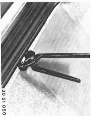
Compress and lift out clips with a pliers.
