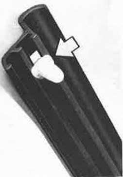
Installation: It applicable, slide on and align new clips.
