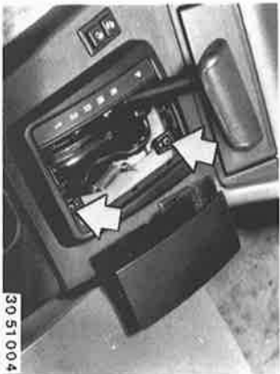
Automatic Transmission: Lift out plate. Unscrew bolts. Remove trim.
