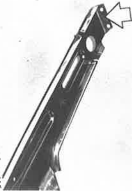
Drill holes for inert gas plug welding at joint between support and wheel house.
