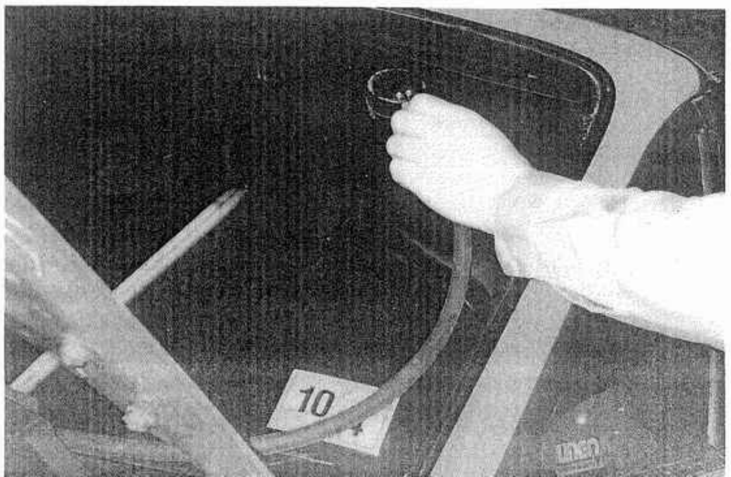
Fig. 18-24. For reasons of safety, the fuel pressure gauge, which is needed to complete the tuning process, should not be placed inside the cockpit. Tape the gauge to the outside of the windshield at a convenient location for viewing while driving.
