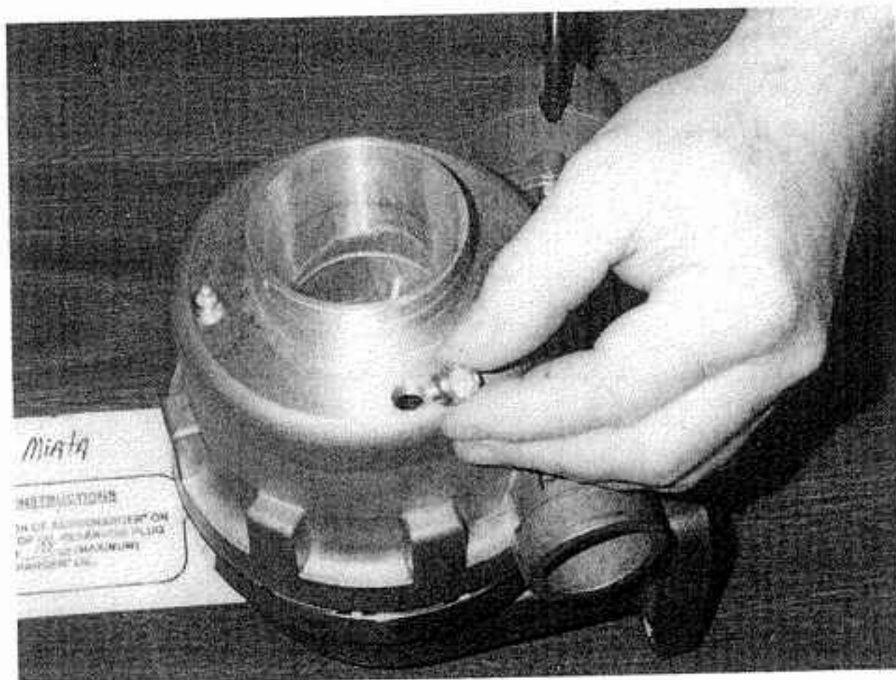
Fig. 18-11. The oil reservoir is sealed with a special sintered brass "breather" plug.
